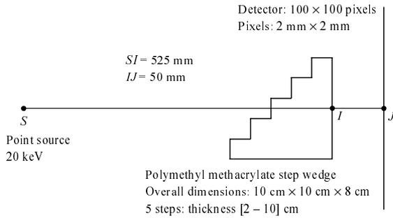
Fig. 2. Geometric arrangement of the simulated experiment. The incident photons are emitted isotropically in a cone with half angle at the apex  $\theta_{\max} = 0.242$  rad. A radiographic image is obtained on the detector placed behind the step wedge (this detector is considered to be perfect). Besides the radiographic image, a dose map is computed in the vertical symmetry plane ( $100 \times 100$  cubic voxels of  $1 \text{ mm}^3$ ).
