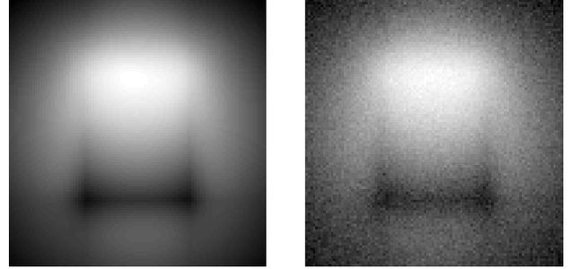
Fig. 5. Simulated image formed by scattered radiation, obtained with the hybrid approach, with  $5 \times 10^5$  incident photons (left) and with the Monte Carlo approach, using  $5 \times 10^8$  incident photons (right). Computation times were about 10 min (hybrid) and 20 h (Geant4), with a 2.8 GHz processor (PC architecture).
