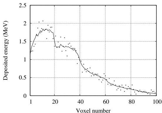
Fig. 12. Profiles corresponding to the 82th column of the detector, obtained with the hybrid approach (solid line) and with Geant4 (dots). The same number of incident photons ( $5 \times 10^8$ ) was used in both simulations.
