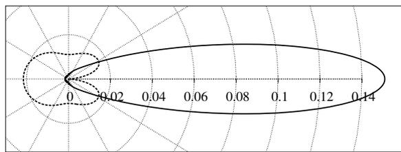
Fig. 4. DCSs for Rayleigh (solid line) and Compton (dashed line) scattering of unpolarized radiation in PMMA, in  $\text{cm}^2 \cdot \text{g}^{-1} \cdot \text{sr}^{-1}$ , computed using the FF and ISF values tabulated in EPDL97.
