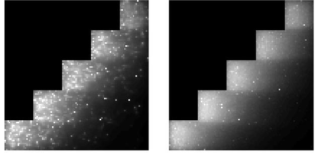
Fig. 9. Energy deposited by scattered radiation, computed using the proposed hybrid approach. The first image (left) was obtained by processing  $5 \times 10^4$  scattering points (corresponding to about  $5 \times 10^5$  incident photons). The second image (right) was obtained with  $5 \times 10^6$  scattering points (about  $5 \times 10^7$  incident photons). Simulations carried out in about 10 min and 16 h respectively (2.8 GHz processor, PC architecture).
