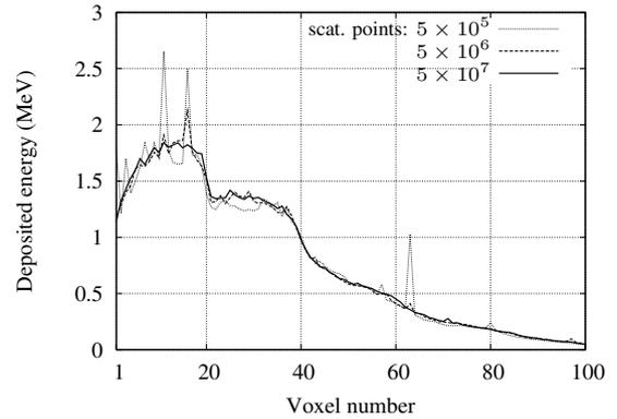
Fig. 10. Profiles corresponding to the 82th column of the detector, obtained with the hybrid approach, with increasing numbers of scattering points, and scaled up to correspond to  $5 \times 10^8$  incident photons. The first simulation ( $5 \times 10^5$  scattering points) took about 25 min, with nearly equal times spent in the two simulation stages. The two other simulations lasted 10 and 100 times longer.
