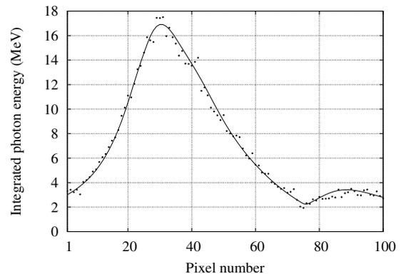
Fig. 6. Profiles corresponding to the 50th column of the images of Fig. 5 (hybrid simulation: solid line; Monte Carlo simulation: dots). The results of the hybrid method were multiplied by  $10^3$  to correspond to the same number of incident photons ( $5 \times 10^8$ ) as in the Monte Carlo simulation.
