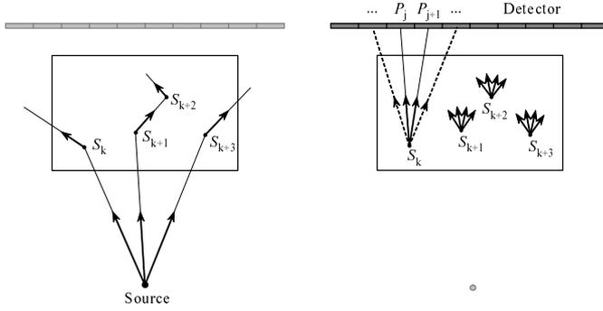
Fig. 1. The hybrid simulation method consists of two stages. The first stage is a Monte Carlo simulation, whose result is a list of scattering events  $\{S_1, \dots, S_k, S_{k+1}, \dots, S_n\}$  (left). This list is used during the second stage, in which scattering is forced towards every pixel of the detector (right).
