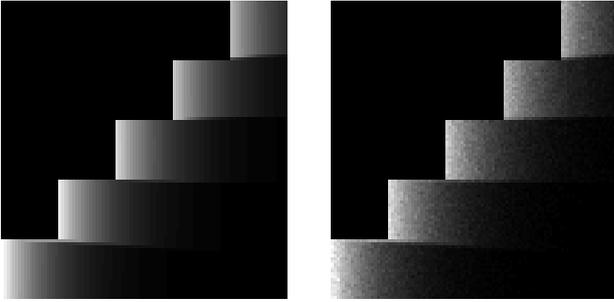
Fig. 7. Energy deposited by direct radiation ( $5 \times 10^8$  incident photons), obtained with the deterministic approach (left) and compared with the results of the Monte Carlo method (right). Computation times were about 1 s (deterministic) and 20 h (Geant4), with a 2.8 GHz processor (PC architecture).
