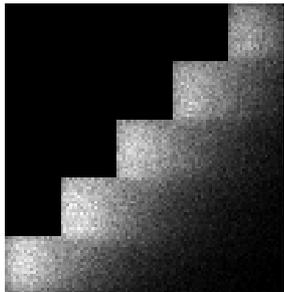
Fig. 11. Energy deposited by scattered radiation, computed using Geant4, with  $5 \times 10^8$  incident photons.
