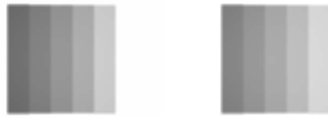
Fig. 9. Two images of Al step wedge were simulated with 80 kVp X-ray spectrum and 7 \times 7 area source in counting mode (left) and energy mode (right). There is not much difference in images, but it shows slightly high contrast in counting mode.
